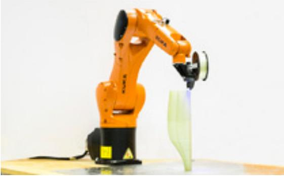
**Robotic arm:** Mechanical arm, usually programmable, with similar functions to those of a human arm. The molten system is placed on the tip which deposits the material but, unlike the other systems, it does not have to be layer by layer.
